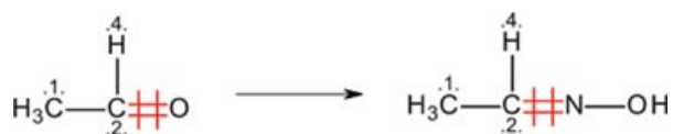
FIGURE 11 | Automapper found the correct AAM and reaction center for this simple, unbalanced reaction. Note: The reacting bonds are marked in red and also with hash marks.
