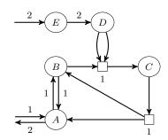
Figure 10: Example of a formally autocatalytic flow using pairs of mutually reverse reactions. Here, the reactions can be ordered such that no two-step futile sub-pathways are present.
