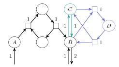
Figure 9: Example for local reasoning of reaction ordering on a seemingly formally autocatalytic flow. In all interpretations of the flow, the violet reactions into and out of D forms a futile two-step sub-pathway. After removing the flow on these reactions we can then apply the same argument to C, and then once more on the I/O flow of B. This leaves the net reaction A  $\longrightarrow$  B.
